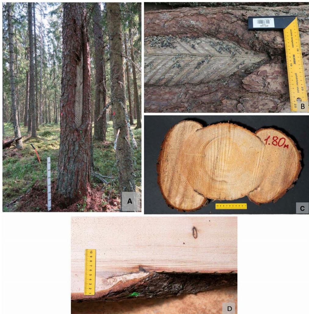
Fig. 1 Sixty-three-year-old resin tapping wounds on 135-year-old stem of Pinus sylvestris (Site 1—Kalsnava); a wound on a standing tree; b close photo of wound surface; note width of scars of approx. 0.5 cm, and “step” between scars of approx. 1 cm; c cross section of
