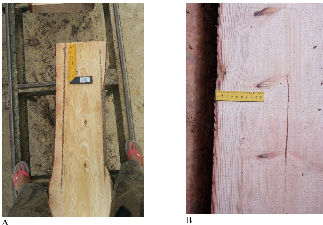
Figure 2.2. Rip-cut of resin tapped P. sylvestris (A) and wood discoloration (B); photos taken by A. Zaluma.
