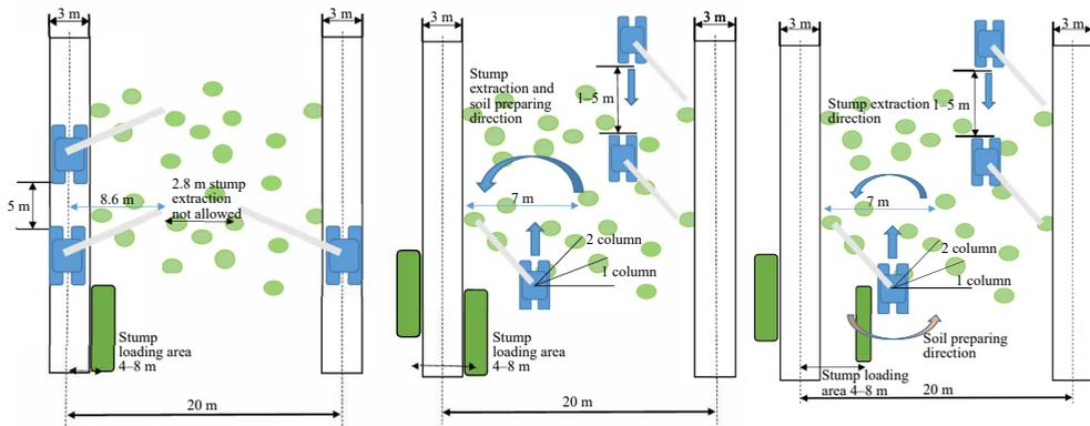
**Fig. 2.1. Work methods for stump-pulling**
