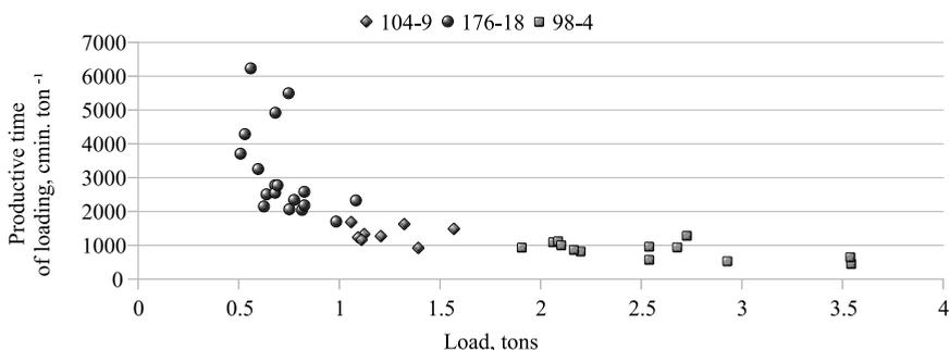
Figure 4. Productivity of loading depending on load size.
