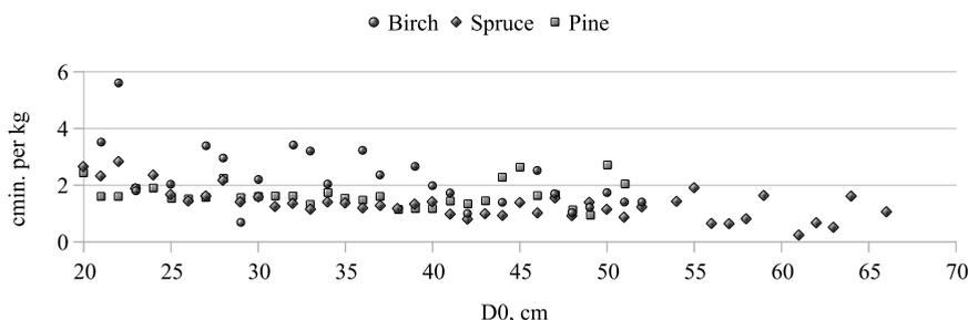
Figure 2. Productivity of stump extraction depending on dimensions of stumps.
