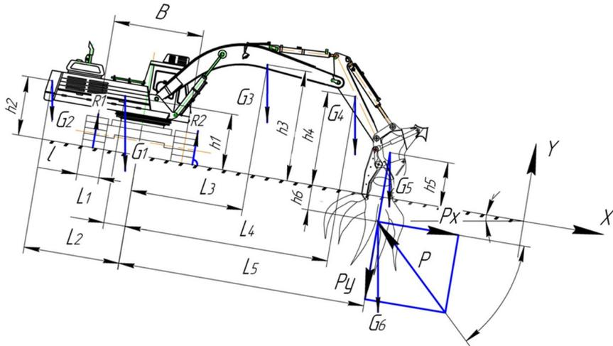
**Fig. 2.2. Force calculations for stump extraction**
