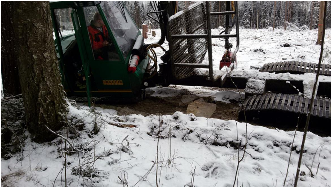
Att. 27: Riteņtraktora risēs iegrimis Logbear F4000 forvarders.
