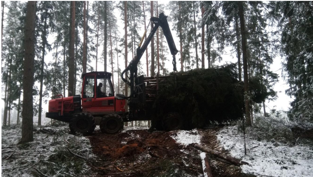
Att. 54: forvarders Komatsu 855 51 .
