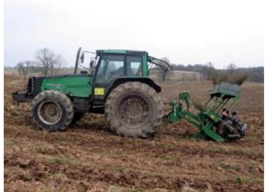
Planting by one or two employees. One of them can control hydraulic distributor and to lift mechanism at the stumps.
