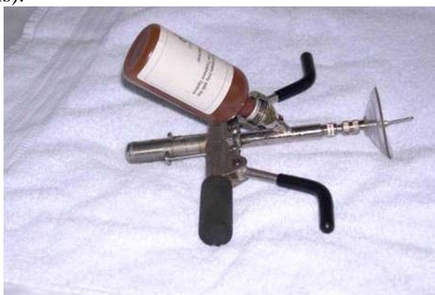
6.3. attēls no Almqvist (2007). The Wedge™ Direct-Inject™ tree injection unit from ArborSystems (Omaha, USA) tested in 504 Ālbrunna.
